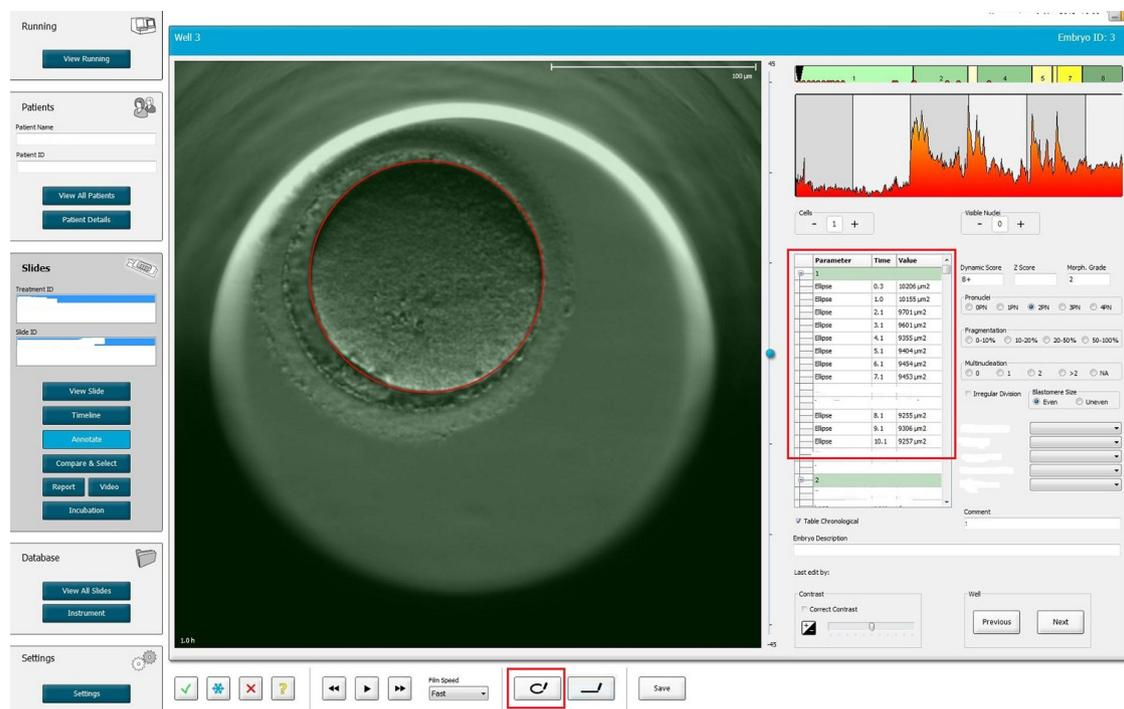
**Fig. 1 – The Embryoviewer® software showing how oocyte elliptical area was measured using the “ellipse” function.**
